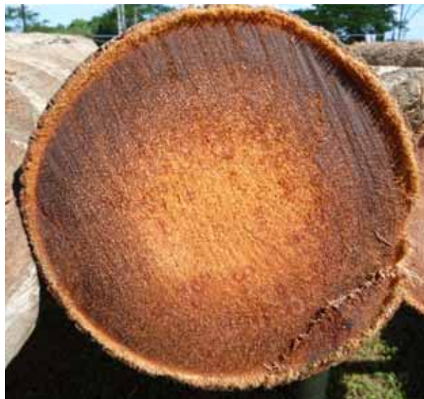
The fibre or 'wood' density decreases towards the centre and with height.
