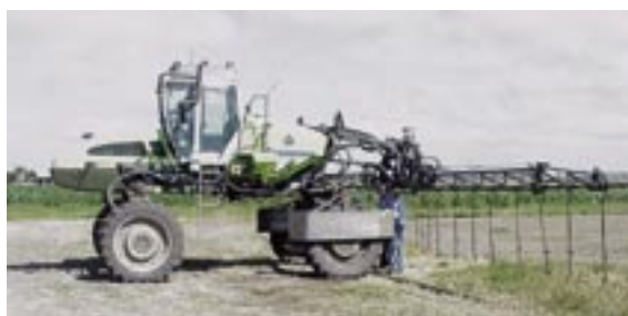
Figure 3. Spray boom fitted with droppers to apply biopesticides in maize (Photo: B. James)
