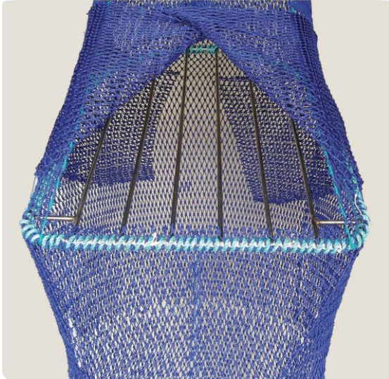
Figure 11a. Rectangular escape opening with double flaps
