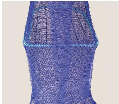
Figure 13b. Double flap configuration
