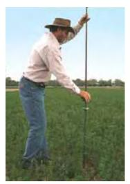
Figure 20: Using a drop penetrometer in the field to measure soil resistance
