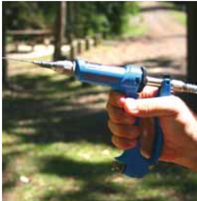
Drenching gun used for splatter technique (Photo: A. Clark)
