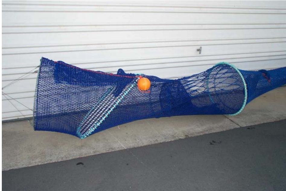
Figure 3.23 The TED and radial escape section BRD that were tested during the 10-day charter in the eastern king prawn fishery in October 2001. The large meshes extend half way around the circumference of the net.
