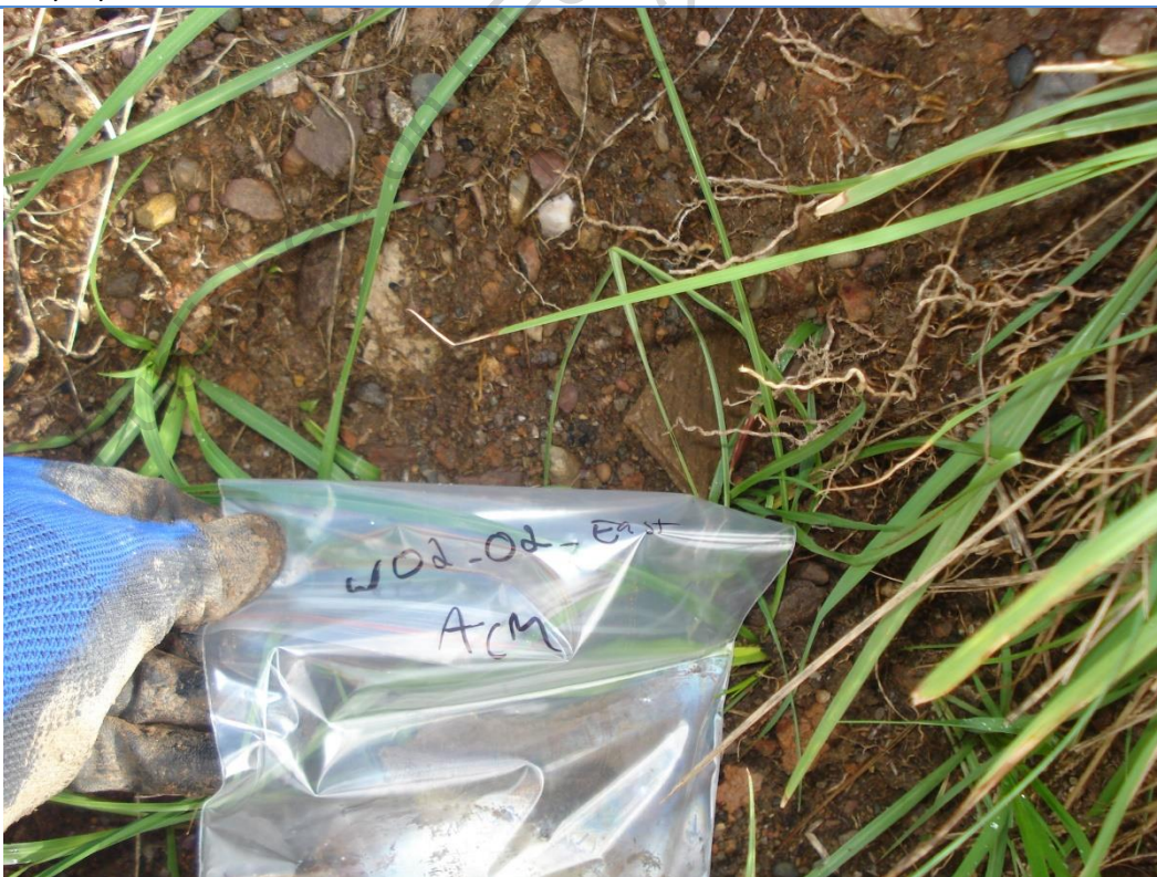
Plate 6 – Bonded (non-friable) ACM identified during field screening at W02_02. Date: 01/04/2021
