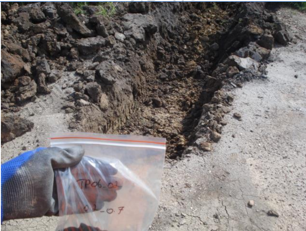
Plate 4 – FILL material observed at TP06 from 0.0 – 0.7 mBGL: CLAY, high plasticity, yellow to grey with brown mottling, wet.
