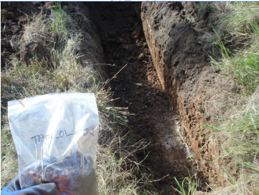
Plate 2 – FILL material observed at TP01 from 0.0 – 0.9 mBGL: CLAY, high plasticity, yellow to grey, moist.
