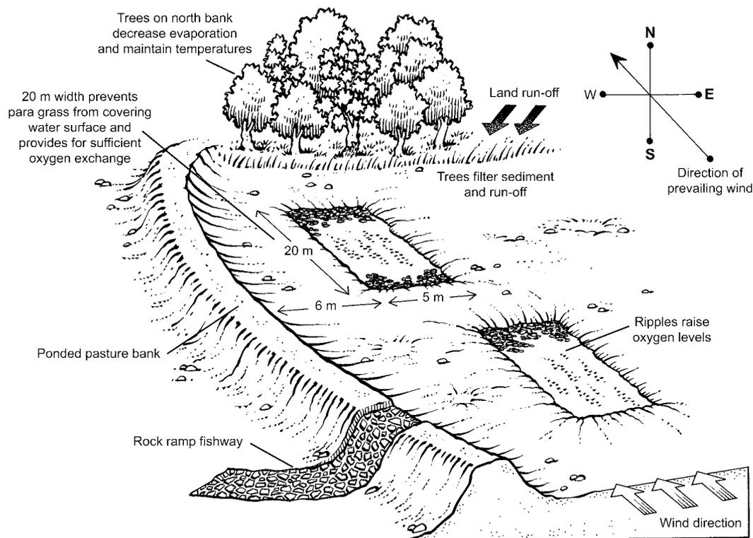
**Figure 3.** Optimal poned pasture layout provides maximum fisheries benefits; note deep water reservoirs and buffer zones.
