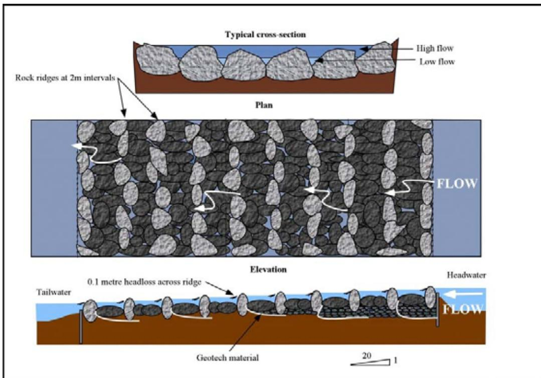
**Figure 2.** General layout of a Rock-ramp fishway.
